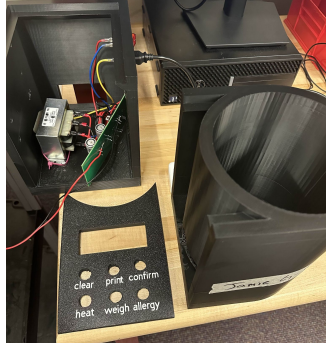
Enclosure w/ Transformer and Rectifier circuit
